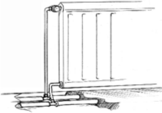
Insulated pipes for the radiator circuit embedded into the floor.
