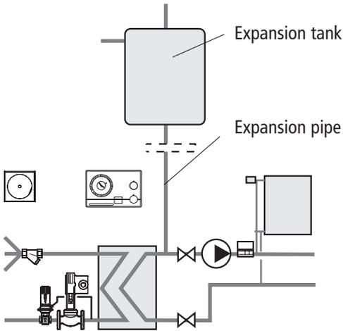
Pump in the flow pipe and no shut-off valve between the heat exchanger and the expansion tank.
