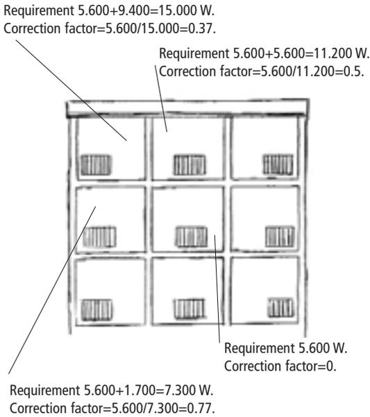
The heat consumption, for apartments of the same size, will vary depending on how many outer wall and roof surfaces there are. A correction factor can be calculated based on the heat requirement per apartment or per square meter.
