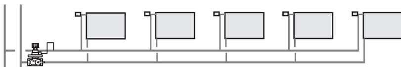
The differential pressure controls give the same available differential pressure to each radiator circuit.
