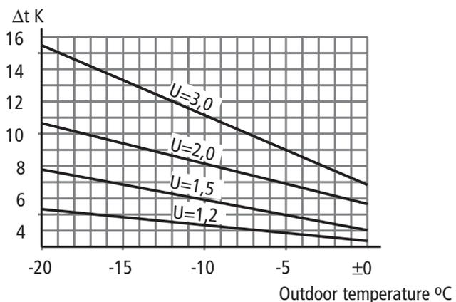
Difference in temperature between room, 20°C, and window of different window constructions. Window temperatures below +12°C can cause radiant cooling. Window with sealed double glazing give a U = 3.0.
