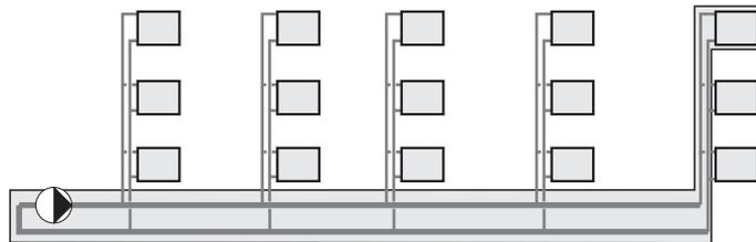
The design circuit is the pipes from the heat exchanger to the radiator located farthest away. The resistance in this circuit is equal to the pump head.
