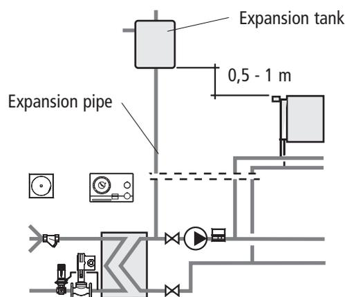
The lower edge of the expansion tank should be placed above the highest point of the system.
