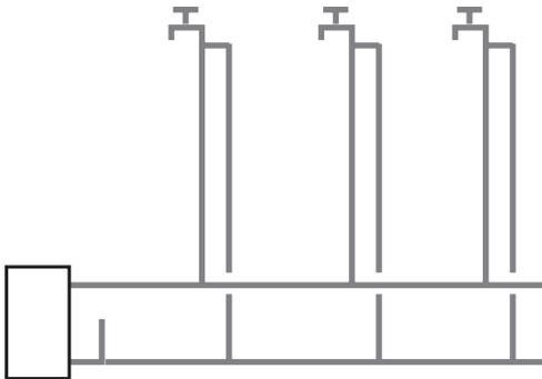
A gravity circulating system makes water of the right temperature available throughout the whole system.
