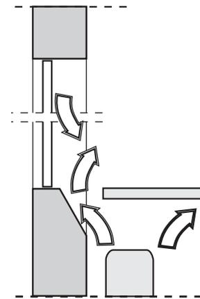
The down draught from the window can be prevented by the heat from the radiator if the window bay and the windowledge are designed properly.
