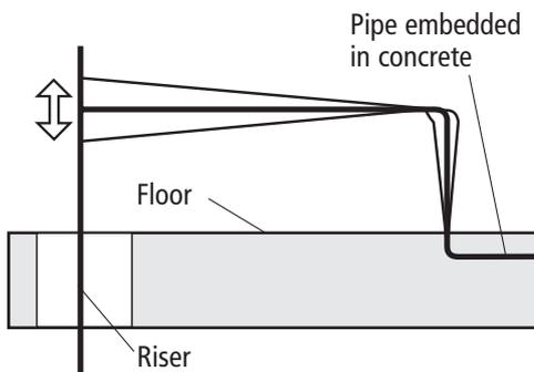
The expansion of the riser must be taken into consideration when the branch is installed.
