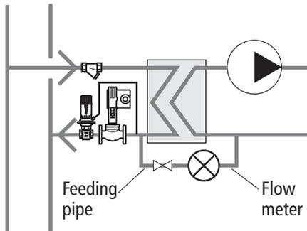
The secondary system can be filled up with treated water from the district heating system but controlled. The amount of water fed into system is to be measured and leakages are not acceptable.
