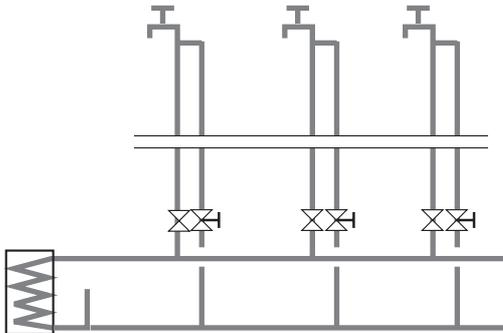
Principles for domestic hot water in installation with circulation pipe, shut-off and adjustment valves.
