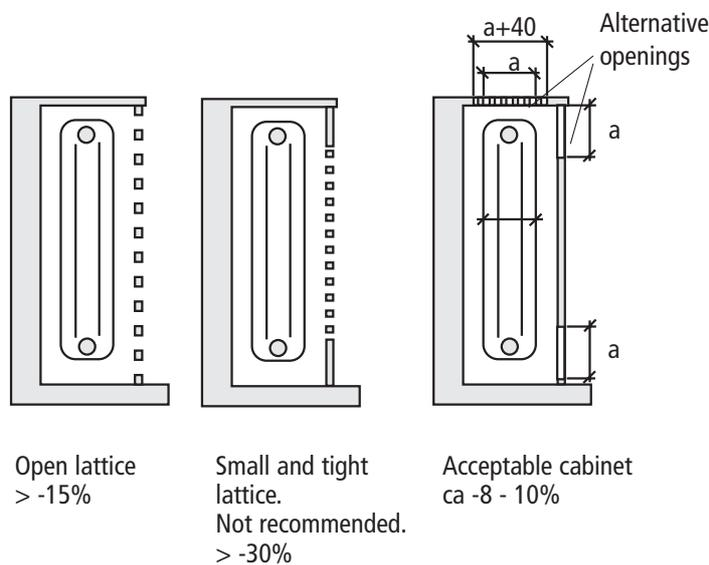
Covering a radiator reduces the heat emission.
