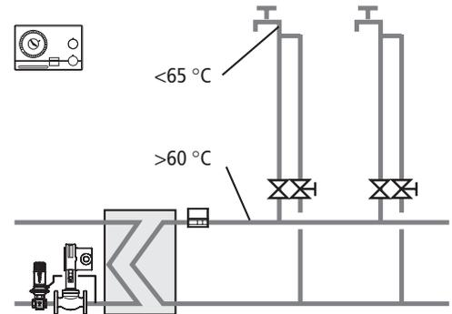
Control of flow temperature for domestic hot water. Maximum and minimum temperatures are important.
